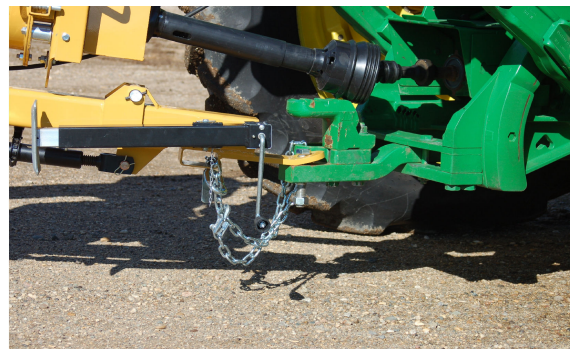
Fig. 4a BOLT AS HITCH PIN
