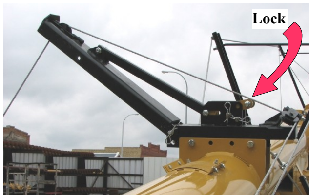
Fig. 15 NEW LIFT ARM MECHANISM
