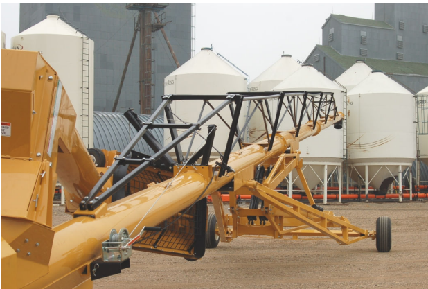
Fig. 5 ALIGN AUGER WHILE IN LOWERED POSTION
